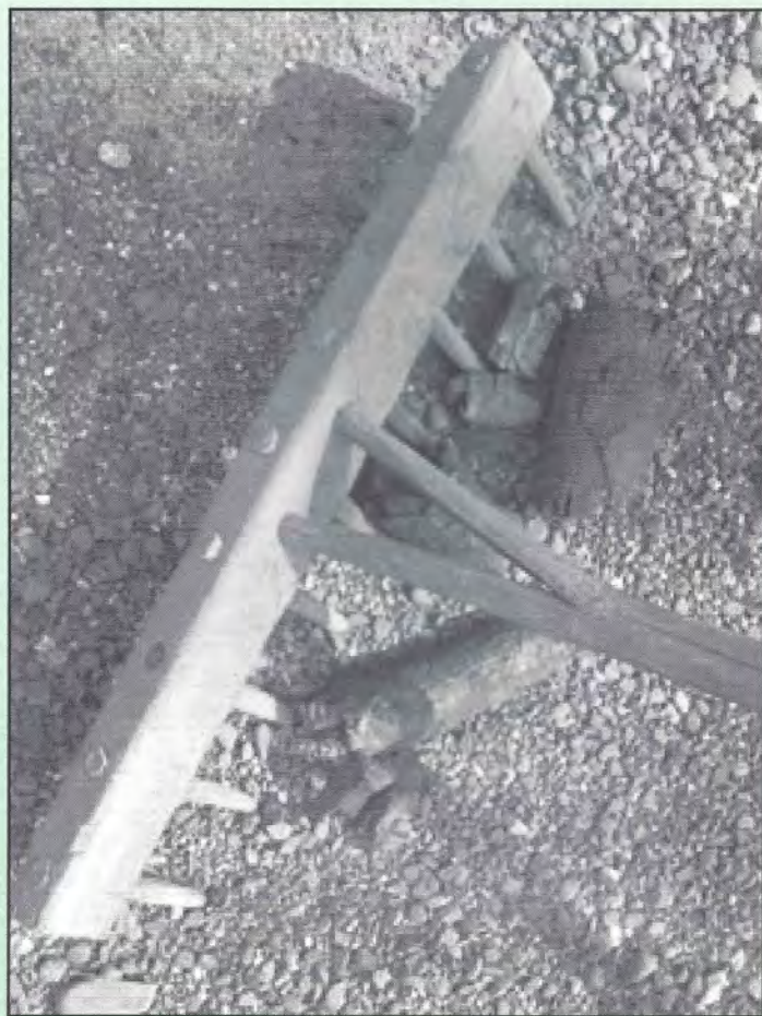
Rake with seven-foot handle made by Guiseppe to spread charcoal to cool after mound was opened.
