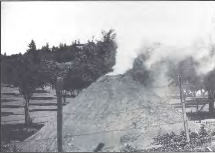
A fire was started inside the center flue of the cone from the top.
