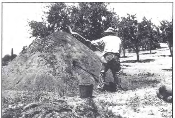
Dirt was piled on top of the pine boughs and packed down leaving a hole at the top. Holes were punched all around the pile from the bottom to about 2 or 3 feet from the top.
