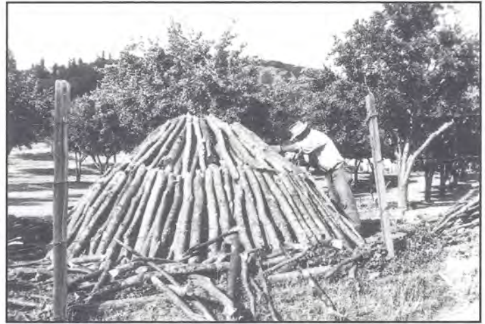
A second tier of oak logs was stacked on top of the first.
