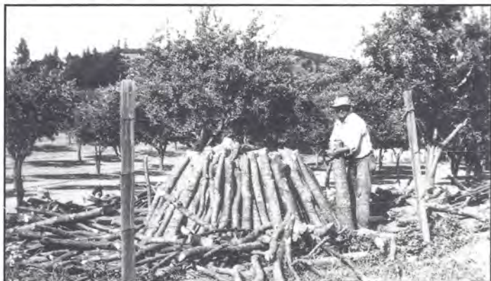
First a flat space of land was cleared. Oak was cut into four-foot lengths and stacked as shown.
