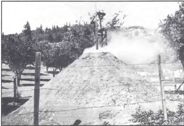
Giuseppe had to stoke (stir and add fuel) the fire to keep it burning. He is standing on a ladder leaning against the cone. Every morning more wood was dropped down through the hole in the top to keep the fire going. Sometimes it was necessary to slow down the burning by putting water down the bole. The pile would burn for 15 days or much longer depending on the size of the pile.
