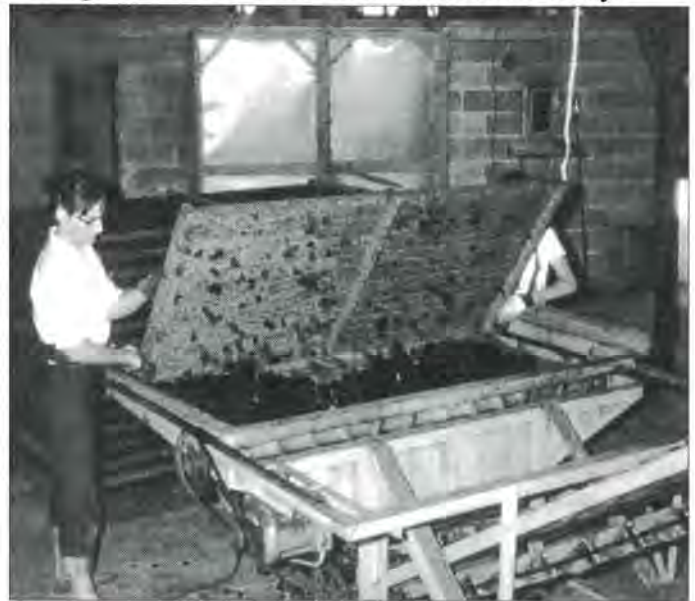
A prune scraper in operation. Diane Schmidt [Carriger], left, Kay Schmidt [Robinson], right. (Note the doors of the dehydrator tunnels in the background.)
